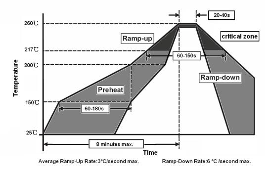
\* Recommended reflow methods: IR, Vapor phase, hot air oven.
